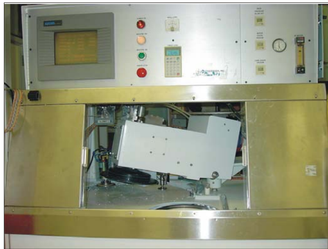
Fig. 1. PadProbe™ installed on the Strasbaugh CMP machine
