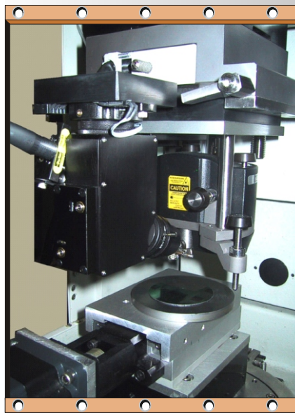
AFM Module Integrated in the UNMT-1 with Linear Stages
