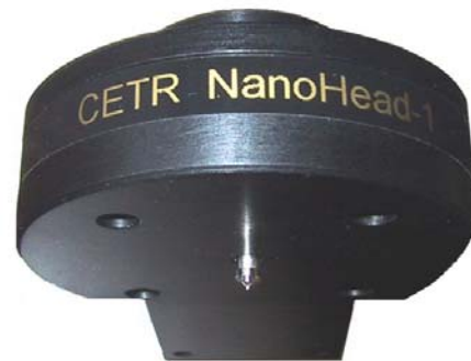
Figure 1: Nano-indentation module for UNMT-1
