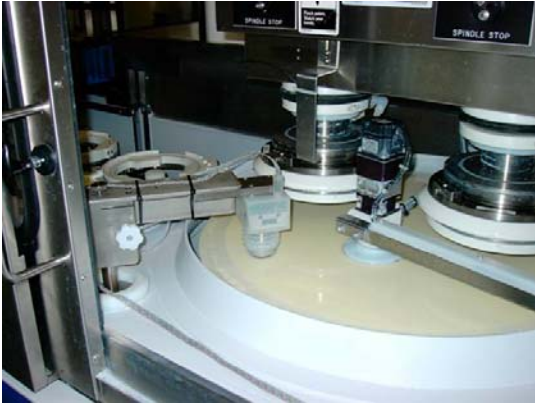
Figure 1. A typical configuration of the CETR Padprobe™. The PP is mounted on an HVM Strasbaugh polisher in this photograph.
